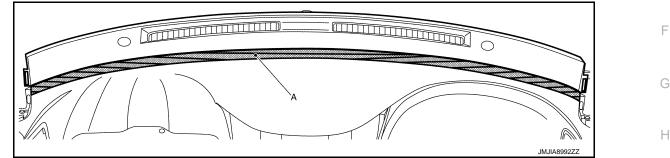
b. Disengage front speaker grille fixing metal clips starting from both sides and work toward the center of the front speaker grille as 1→2 as shown in the figure.
