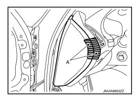
b. Pull instrument side finisher LH, and then disengage pawls using a remover tool (A) according to the numerical order  $1\rightarrow 2$  as shown in the figure.
