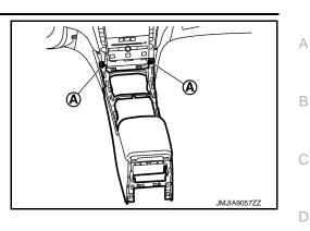
11. Remove the following part after removing center console assembly. Rear ventilator grille. Refer to VTL-12, "REAR VENTILATOR GRILLE : Removal and Installation".
